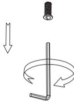
Loosen the hexagonal machine screws of the reflector with a hexagonal wrench and remove the reflector
