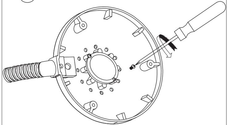
Loosen the screws with a screwdriver
