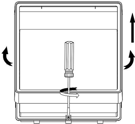
Loosen the screws on the cover and open it
