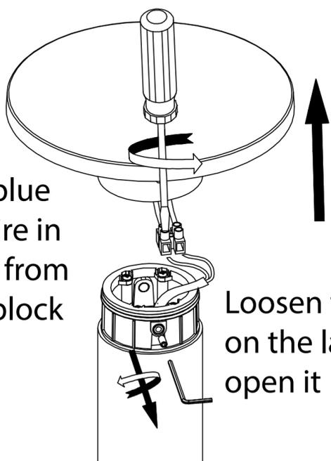
Loosen the screws on the lamp and open it
