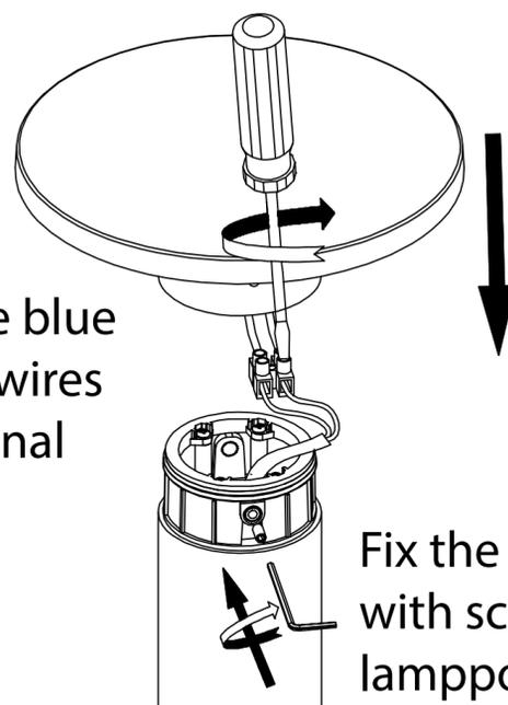
Fix the lamp with screws to the lamppost
