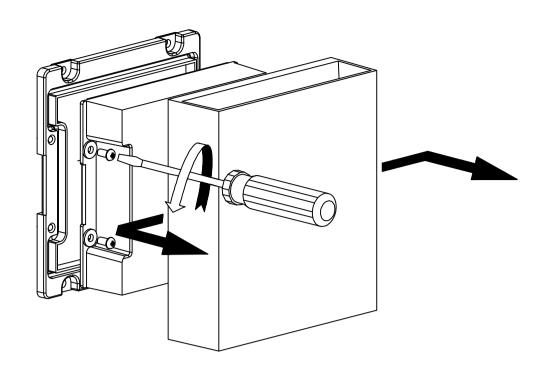
Loosen the screws on the driver. Take out the LED module from the PC cover module.
