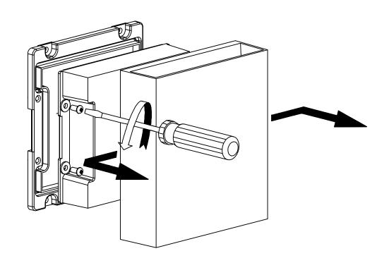
Loosen the screws on the driver.
