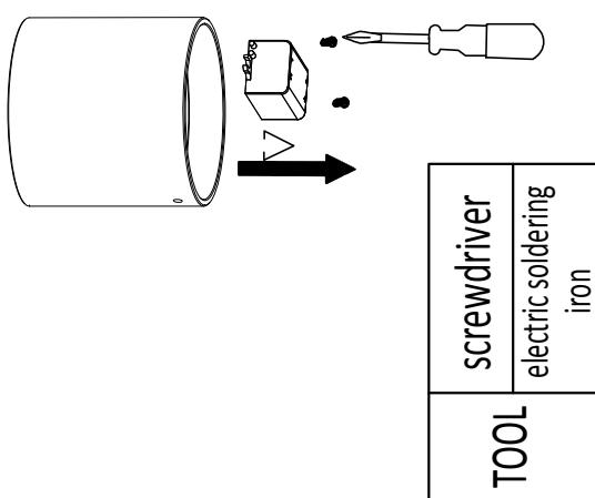
**A** remove the hexagon screw to open the device
