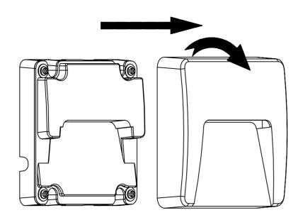
Loosen the screws on the inner and outer PC cover
