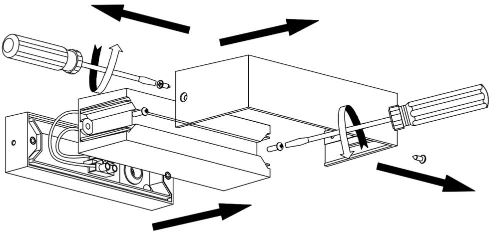
Loosen the screws on the lamp cover and open it
