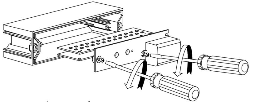
Loosen the screws on the driver and driver holder
