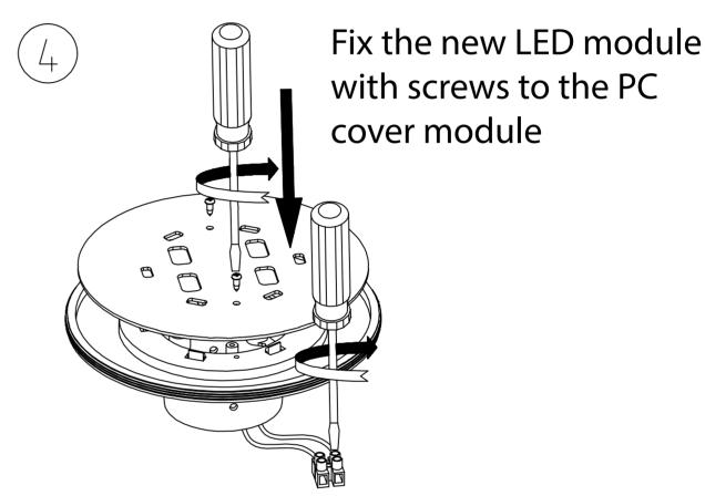
Connect the blue and brown wires to the terminal block
