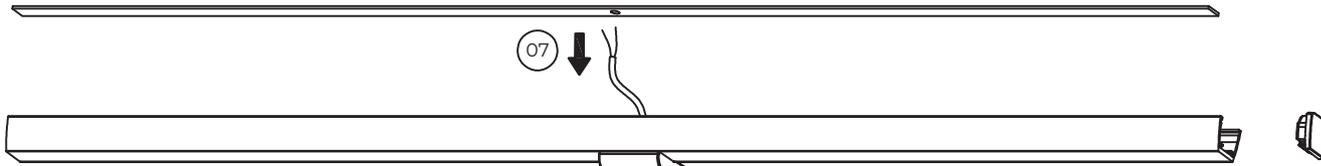
03 Loosen the wires on both sides (blue and brown wires) using a tool. Then change the driver and re-connect the wires on both sides.
